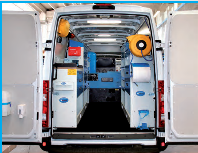
Iveco Daily with storage shelves, provided with 15 Kwa generator and compressor.
