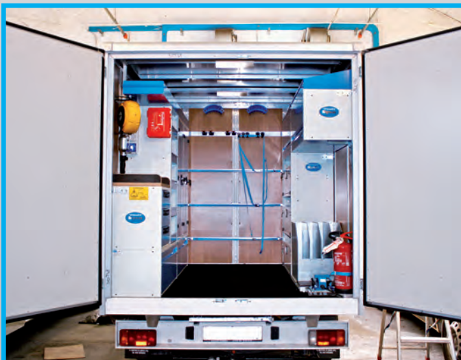
Mobile workshop conversion on a small truck.
