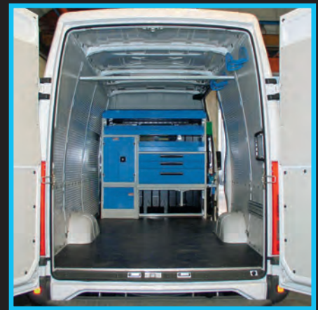
Iveco Daily: a van upfit with storage units installed against bulkhead
